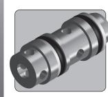
The SV25C is a cartridge shuttle valve. The valve will the higher of two pressures and send this oressure to the outlet. The valve often used to provide redundancy on pilot systems. In the event of pressure loss on one inlet, the valve will automatically switch to the higher pressure supply.
