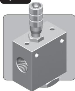
The CMF75 is a 3/4" nominal bore metering valve with a reverse free-flow check function. It provides metered flow in one direction, and free flow in the opposite direction, ideal for uni-directional speed control of a cylinder or actuator.
