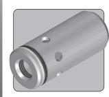
The CC50 is a 1/2" nominal bore cartridge check valve. It will allow flow in one direction, and blocks flow in the opposite direction. It may also be referred to as a non-return valve.
